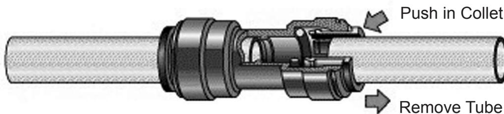
Push tube firmly into the fitting connector all the way until the tube stops. Try to pull the tube out to check the security. If the tube pulls out, then push all the way in again.
